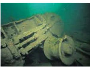
Further images from JEL; spooked agricultural wheels, piles of which can be found throughout the wreck, left, and cargo winch upside-down in the second hold, showing a small steam engine driving the winch, right.
